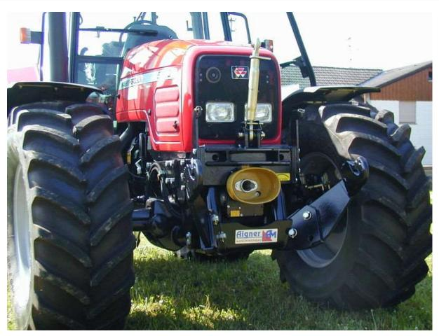
SERIES 8400 Front linkage: lifting force 42 kN
