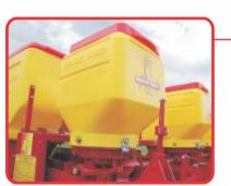
**Seed Bin:** polyethylene bucket type for thick grains, with 25 kg capacity per row.
