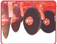
**Seed sowing:** the seed sowing system is thought two mismatched disks mounted in "V" shape with 13" and 14".
