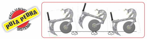
Feeling the need of several producers who cultivate rocky lands, VENCE TUDO has developed the most efficient penetration and ground attack system. Baptized and patented "stone Jumper" a simple name which exemplifies in a practical way it is essential operation to a uniform and much more efficient planting, ensuring better germination and significantly avoiding breaks and stops, common in these soil situations, reducing time and costs in the plantation process.
