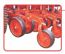
**Cover mechanism:** two rubber wheels for depth control and 3rd compactor wheel.
