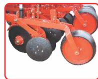
**Option:** Two small disks, system for cover up the row, with compactor and depth control by 3rd wheel.
