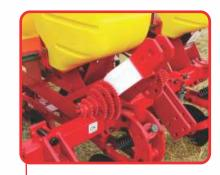
**Transmission Adjustment:** by a combination with sprockets, the sprockets are fixed in the easy place in the frame.
